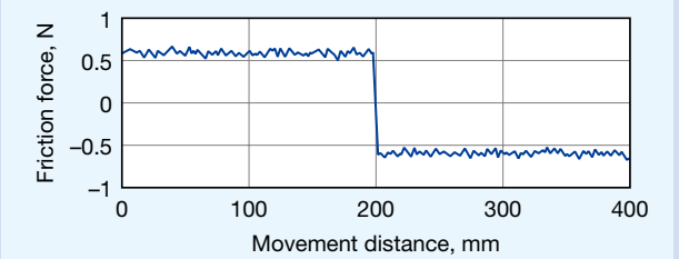
Fig. 1-1 Fluctuations in dynamic friction
